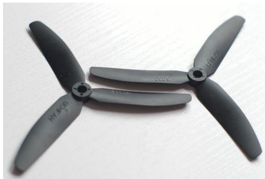
Figure 5. Propellers 5030 R for the UAV
