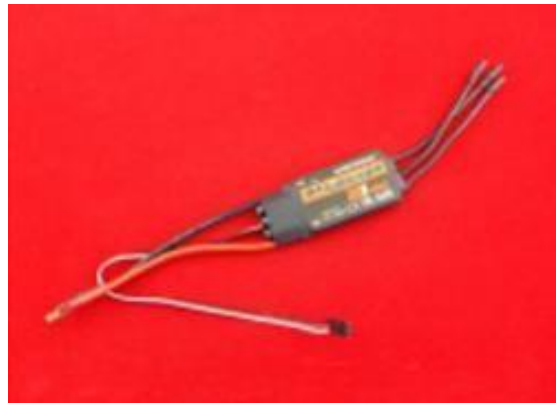
Figure 7. Electronic Speed Controller 60 A
